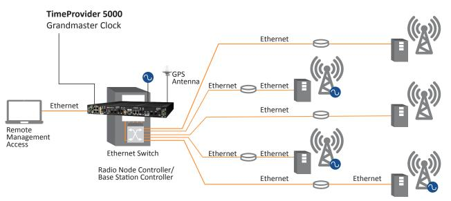
Typical wireless backhaul application utilizing the TimeProvider 5000 Grandmaster Clock with fully redundant, carrier-class architecture to provide precise timing and frequency for remote base stations over a packet-based Ethernet network infrastructure.
